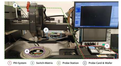
1 PXI-System 2 Switch-Matrix 3 Probe Station 4 Probe Card & Wafer
